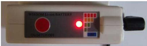
2. Press ON/SETUP/OFF again when the LED turns orange, the output power is around 75% and the temperature reaches 40°C-45°C.
