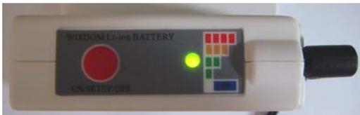
4. Press ON/SETUP/OFF for the fourth time when the LED flashing, it is in the model of power saving.
