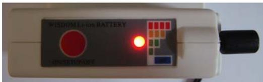
3. Press ON/SETUP/OFF for the third time when the LED turns green, the output power is around 50% and the temperature reaches 35°C-40°C.
